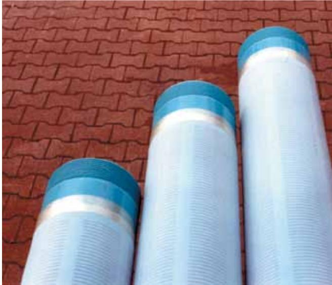
These casings withstand external pressure loading which is caused by geological formation, the depth of the groundbed, the ratio of borehole diameter to casing diameter and the position of dynamic water levels.
