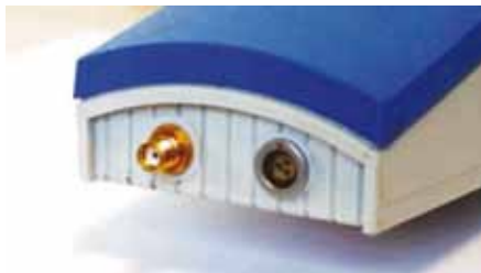
DCF-77 and GSM antenna terminal
