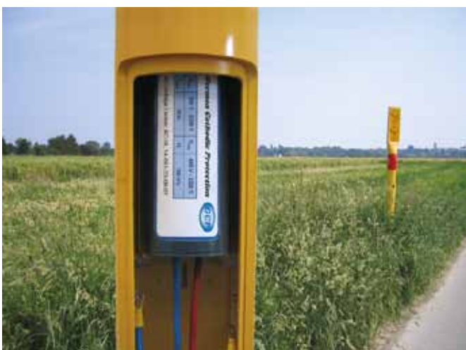
The dimensions of VL-14-401 allows installation inside test stations
