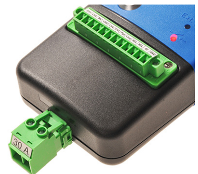
4 DC and 4 AC Inputs 30A relay for switching rectifier regulation
