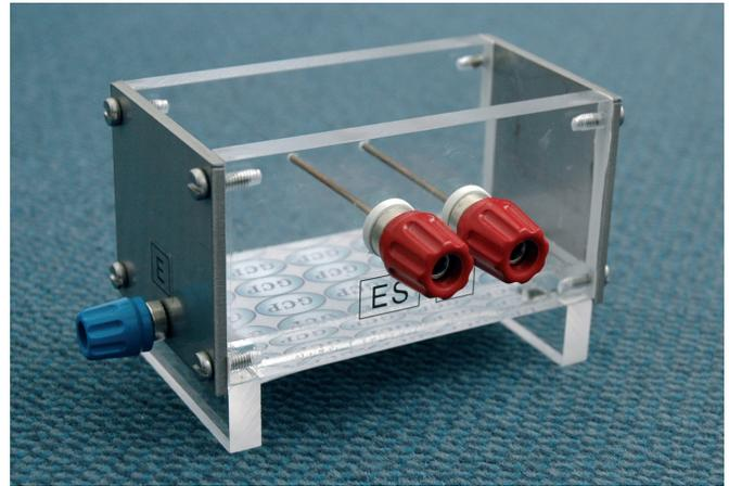
The soil box can be used for the measurement of specific resistivity of electrolytes ie. soil sample, water and conducting fluids.
