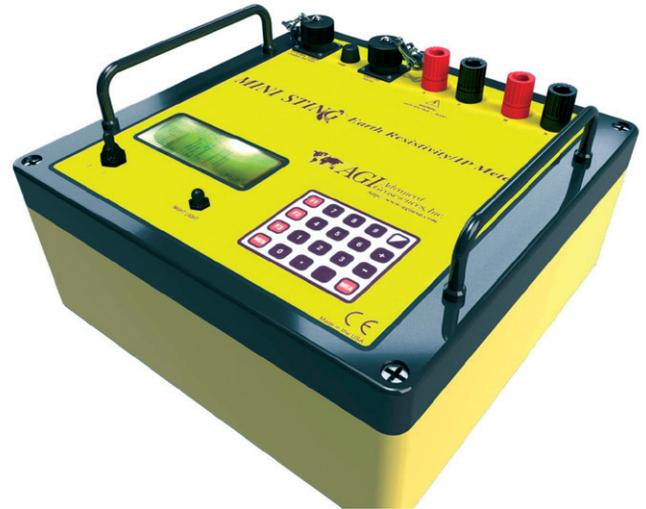
The MiniSting is a high powered resistivity & IP meter especially designed for manual resistivity jobs like electrical grounding-grid testing, the IEEE fall-off-potential method, ASTM G57 soil resistivity test using the Wenner four electrode method, survey for corrosion control, electrical surveys with the four electrode method (vertical electrical sounding or profiling).
